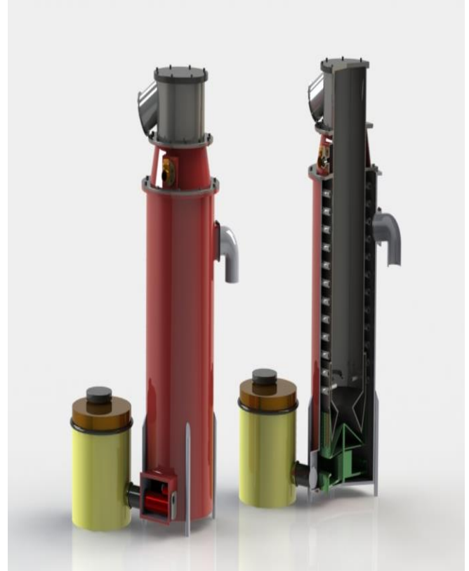
Fig. 1. Schematic of fixed-bed downdraft gasifier.
